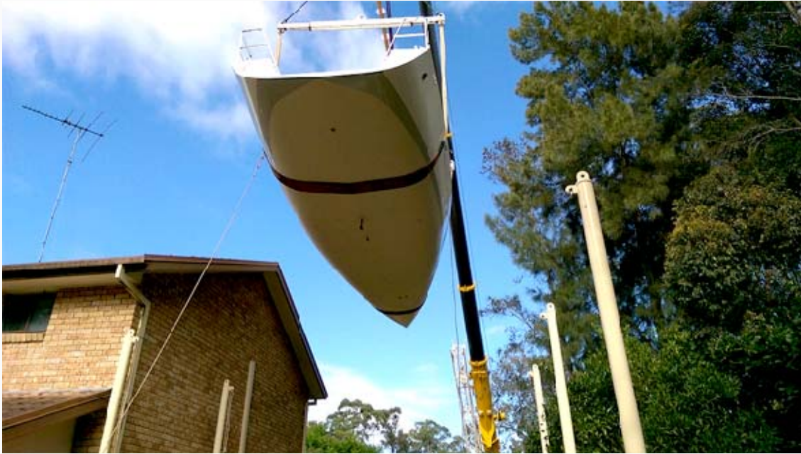
Passion X being lifted to have the keel attached
